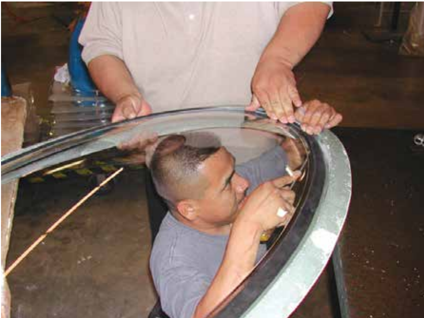
Figure 16 Installing the mock-up acrylic window in a mock-up fiberglass frame made by Mr. Donaldson at Planet Plastics, Corona, CA, May 22, 2003. Source: Donaldson.
